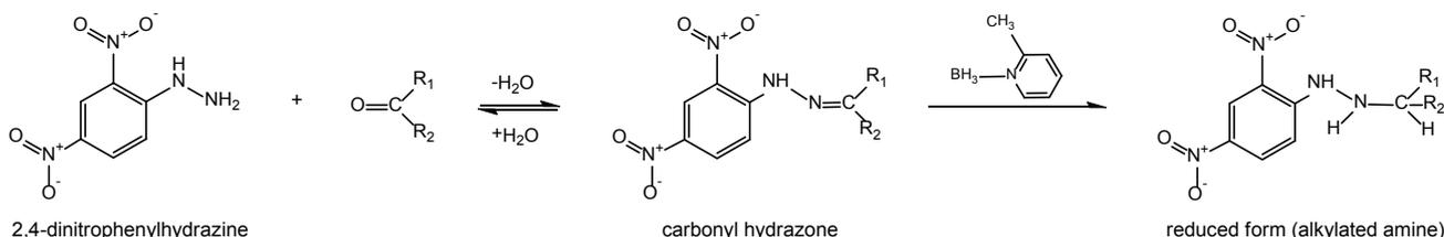
**Scheme 4. Scheme of the reductive amination of carbonyl 2,4-DNPhydrazone with 2-picoline borane.**
