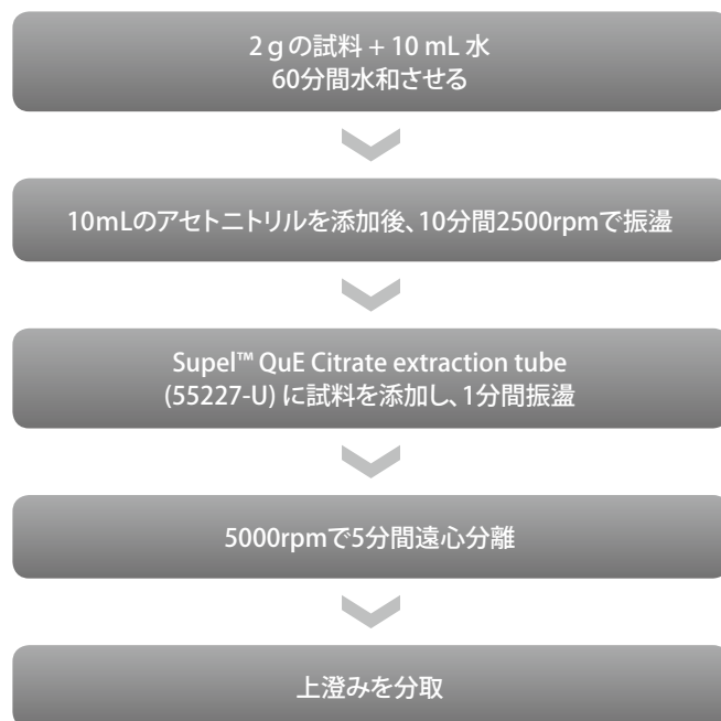
図1. QuEChERS Extraction Procedure Used for Green Tea
