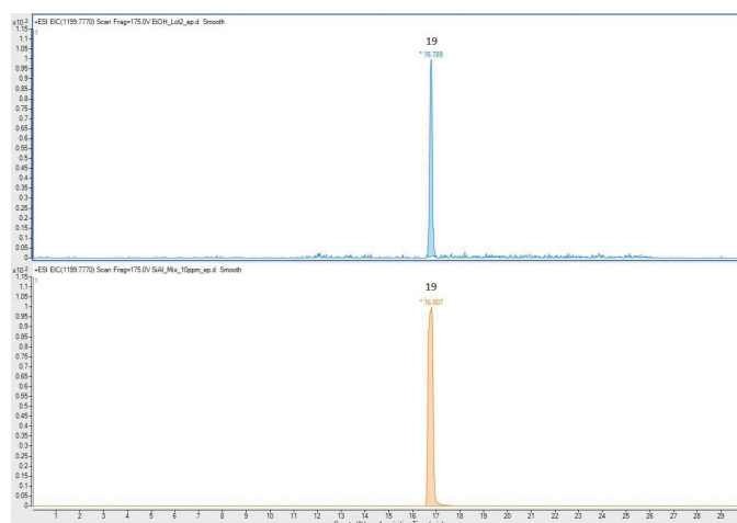
図4. Representative sample of a single-use equipment extraction. Top: Extract Sample of Single Use Filter with 50% Ethanol, bottom: Extractables and Leachables Screening Standard for LC
